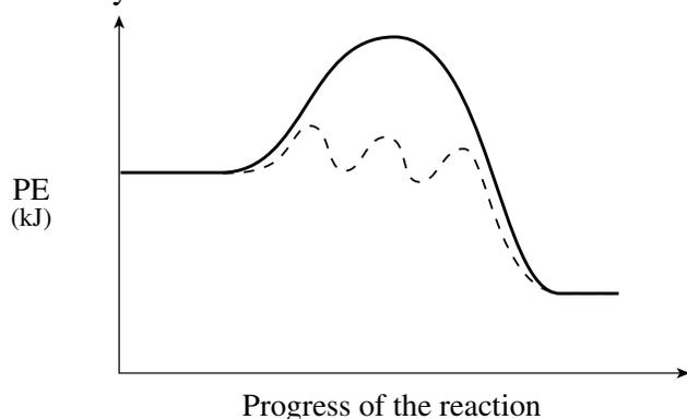
←  $\frac{1}{2}$  **mark** ( $E_{a(\text{catalyzed})} < E_{a(\text{uncatalyzed})}$ )
